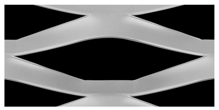
LW Pitch:200.00mmStrand Width:21.00mmSW Pitch:70.00mmThickness:3.00mmWeight:4.86 kg / m2Open Area:40%
